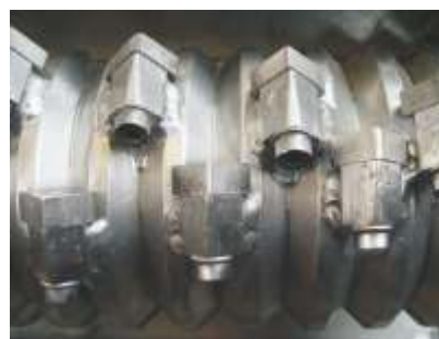
Profile rotor with welded knife carriers (GAZ 62 S)
